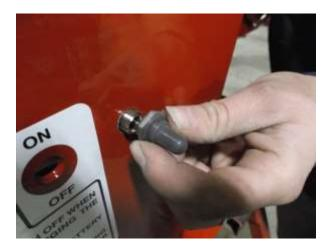
Step 2: Install the actuator switch in the hole and tighten.
