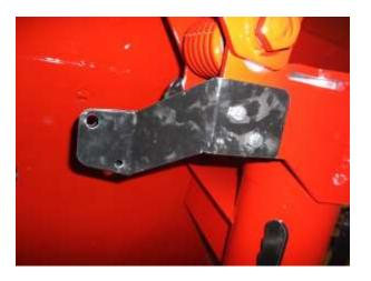
Step 4: Install the Lower Actuator Bracket. The second bracket will be placed towards the outside of the trailer and the bend angle is towards the centerline of the auger tube. Attach using 2 -3/8" x 1-1/2" bolts, 2 - 3/8" lock washers, and 2 - 3/8" nuts. Tighten all fasteners. Make sure actuator mounting holes align.
