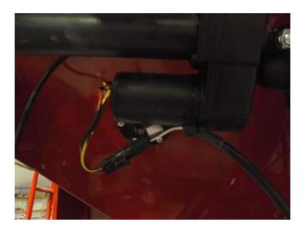
Step 9: Use a single zip tie to hold the cord to the actuator motor.
