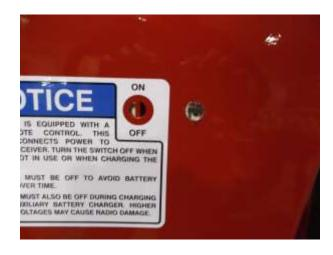
Step 1: Drill a 1/2" hole next to the "ON/OFF" switch hole.
