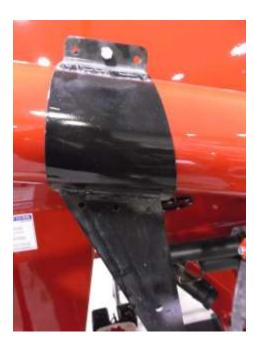
Step 6: Rotate the actuator up to get an idea of where to place the Top Actuator Bracket assembly. Use 1 - 5/16" x 2-1/2" bolt, 1 - 5/16" lock washer, 1 - 5/16" nut to hold the two sides of the Top Actuator assembly together. Make sure to place all nuts towards the outside of the tender.
