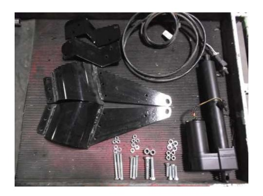
Parts required to install a 220 Auger Lift
