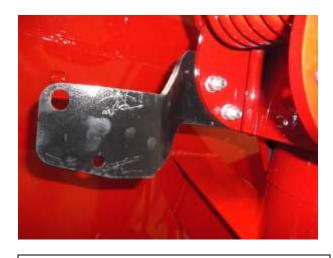
Step 3: Install the Lower Actuator Bracket. The first bracket will be installed next to the hopper body. The bracket should be installed so the bend is towards the centerline of the auger tube. Attach using 2 - 3/8" x 1-1/2" bolts, 2 - 3/8" Nuts, and 2 - 3/8" lock washers. Tighten all fasteners.
