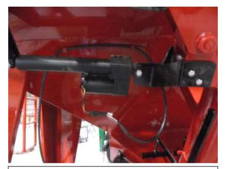
Step 8: Connect the weather pack connectors together. Leave some slack in the harness and route the harness along the side of the tender. Keep harness in place using wire ties.
