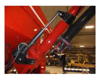
Step 12: Unlatch the auger hold down so the auger is free to move. Makes sure all fasteners are tight, no leaks, and that the wiring harness will not be pinched during raising and lowering. Test the actuator by raising and lowering the auger. Repair any problems if any.
