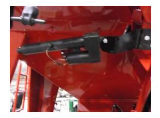
Step 5: Install the actuator into the pair of lower actuator mounts. Use a 1/2" x 2-1/2" bolt and a 1/2" nylock nut to fasten the actuator on. Make sure to install the bolt and nut with the nut to the outside of the tender. The nut should be facing away from the hopper to prevent any interference.
