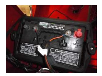
Step 11: Connect the positive fused wire to the positive terminal on the battery. Connect the negative wire to the negative side of the battery. Tighten the connections.
